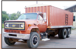
79 Chevy Gas engine tag box and hoist
